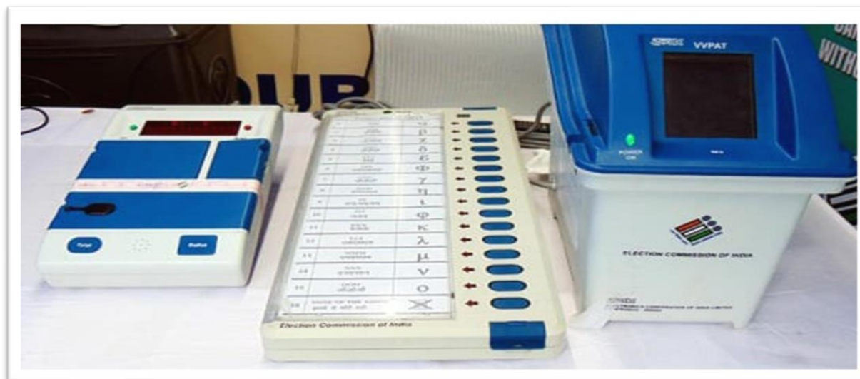
. Figure IX:EVM + VVPAT set-up used in India
